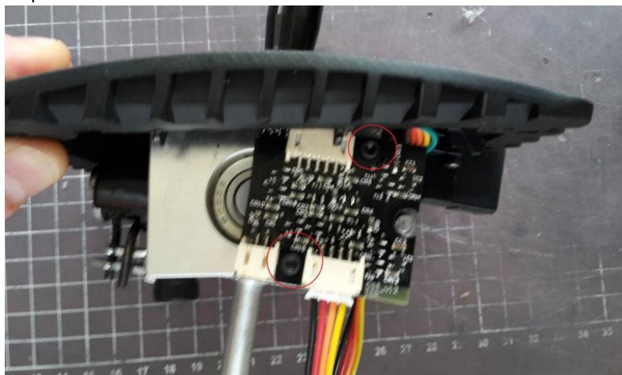
Step 4: Check if all cables are undamaged and plugged in correctly
