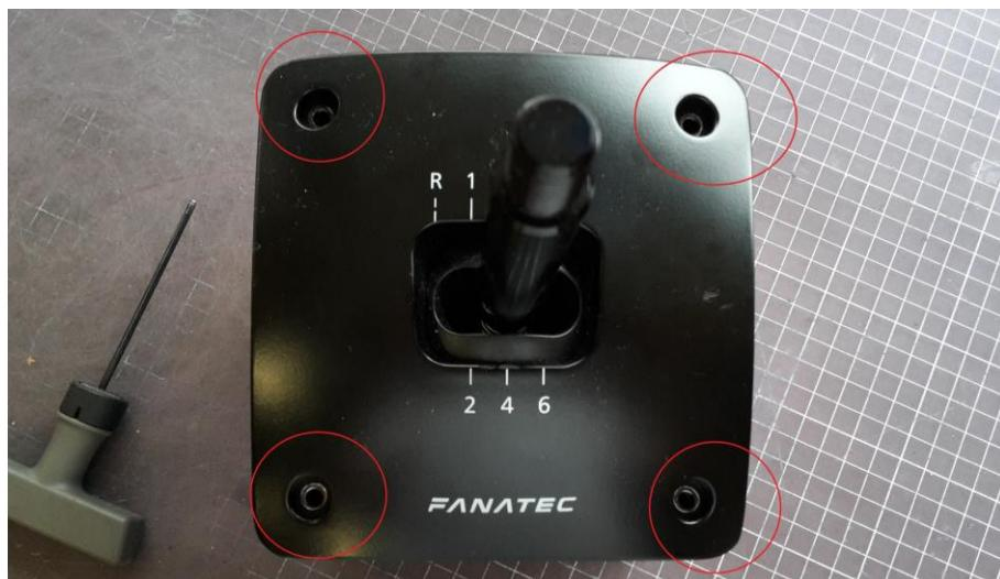
Step 2: Carefully lift the top and unplug the cable, coming from the bottom
